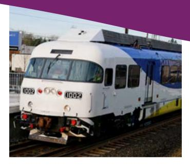
Four cars were purchased from Colorado Railcar for the project: three single powered cars and one trailer car. Powered DMU cars accommodate 74 seated passengers and trailer cars have 80 seats. With the ability to move along the track in either direction, the single-powered cars have cabs at both ends of the vehicle, and the trailer car has a cab at one end only. Both types of cars have room for two mobility devices and up to six bicycles.
